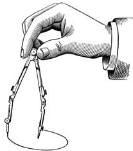
Drawing a circle with a pair of compasses.
